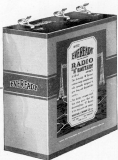
Eveready "B" Battery No. 772 for detector and amplifier. Connections at 22½ and 45 volts. Three Fahnestock Clips. Approximate over-all dimensions, 8¼ in. x 3¼ in. x 7¾ in.
