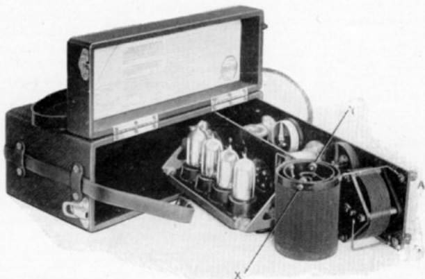
Right: A second case, of the same dimension as that for the batteries, houses the receiving equipment. Notice how the panel swings out to make the sockets accessible. The tube socket unit is mounted on shock absorbing springs to eliminate microphonic noises.
